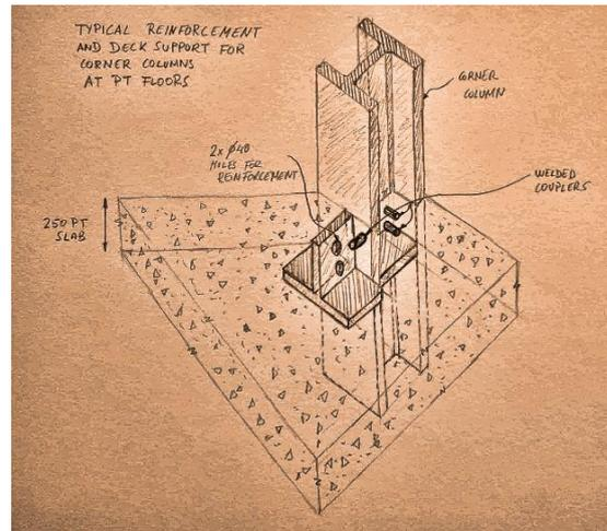
Figure 5. Corner slab support at PT level.
