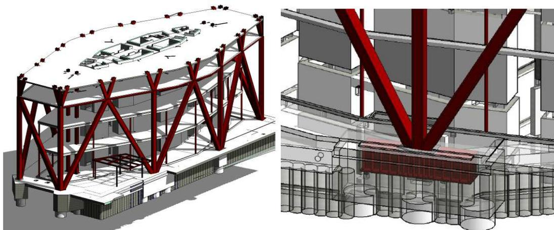
Figure 4. Mega-dia-grid from GF to Level 3 (left) and concrete encased grillage (right). Source: WSP Revit model.
