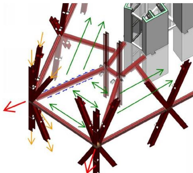
Figure 7. Load path of tying action at node floor types. Source: WSP Revit model
