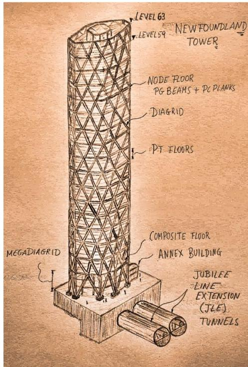
From Level 03, every fourth floor is a node floor which has a different structural configuration compared to the three intermediate floors underneath it.
