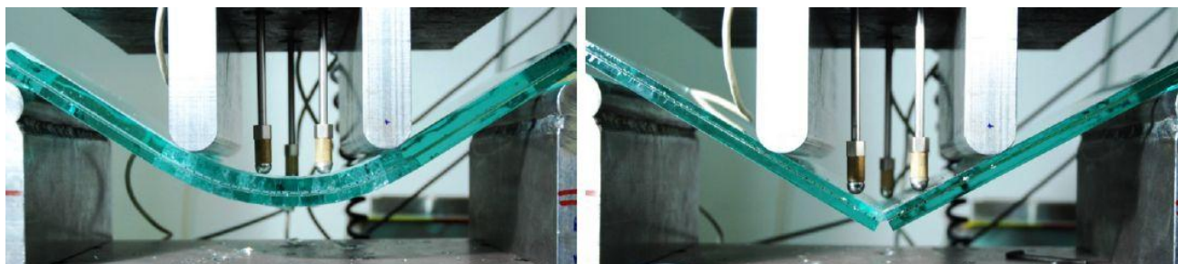
Experimental investigations on post-fracture performance of laminated glass
