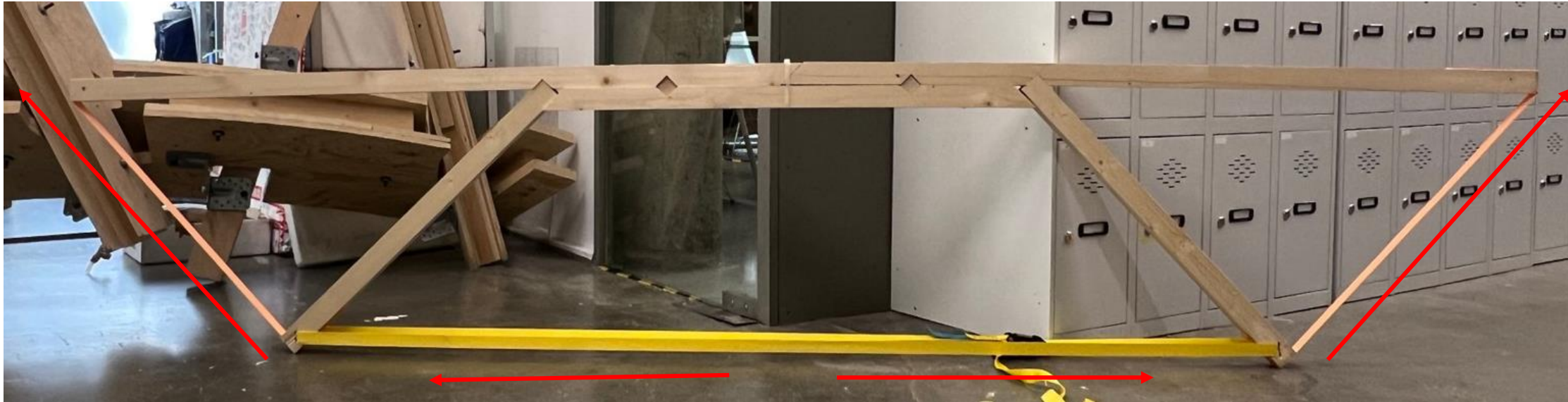
Truss on 1 plane Working on tension connected by ratchet belts
