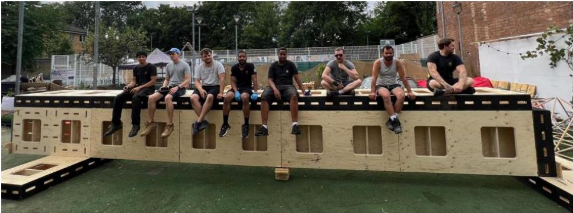
Fig. 9 Test 2 – support spanning beam Somerset House structure – THIS BRIGHT LAND
