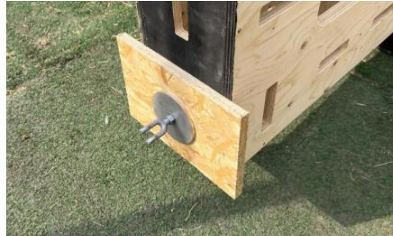
Fig. 10 Cable within block to provide tensile capacity at bottom of the beam
