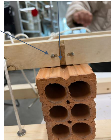
Dowel functioning as a shear key
