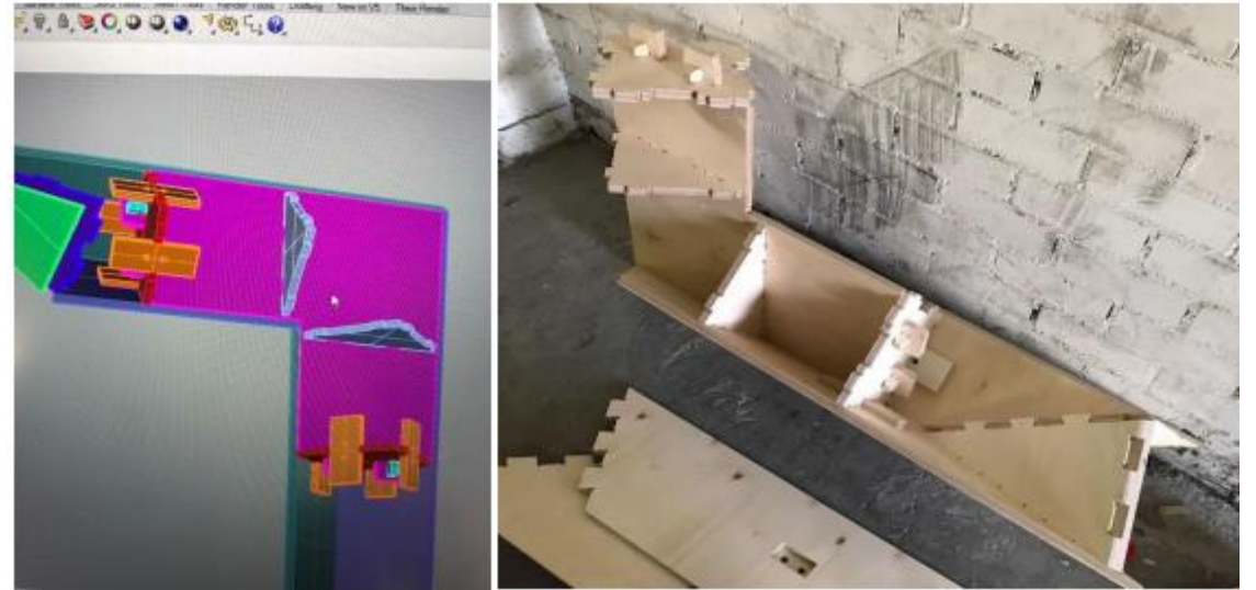
Fig. 10 3D digital model + physical 1:1 of the knee part internal cross section
