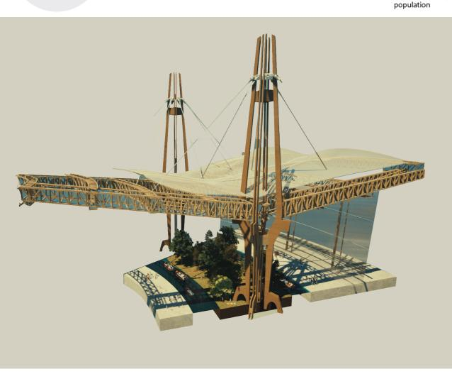
Timber is used instead of steel as it is a renewable material with a lower carbon footprint and is well-suited to prefabrication, allowing for efficient on-site assembly. Beyond its structural and environmental benefits, exposed timber surfaces contribute to a warm, natural aesthetic that enhances occupant comfort and creates a more welcoming, human centred environment.
