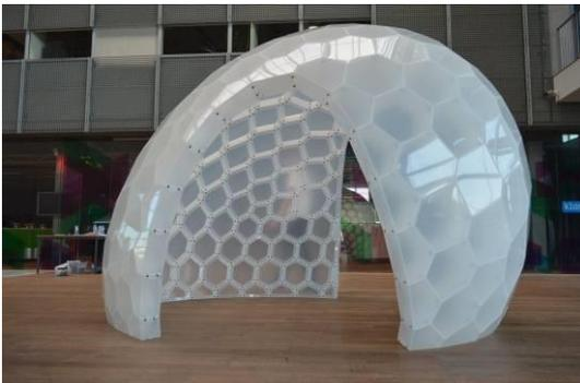
Figure 1: Polypropylene shell pavilion structure
