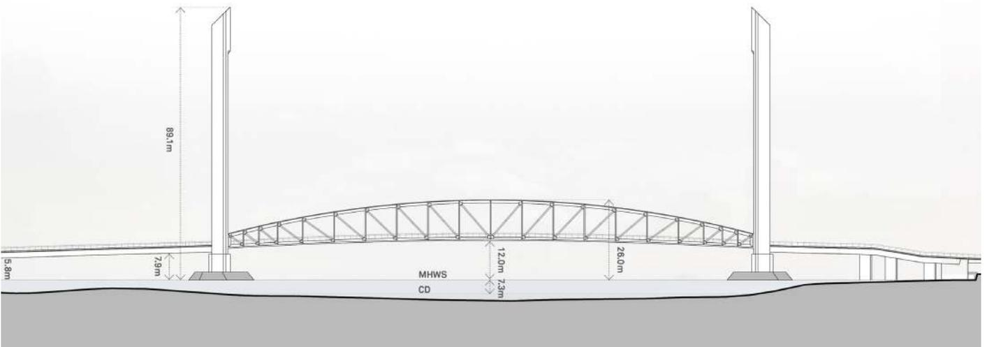
Figure 5 - Elevation of the Rotherhithe to Canary Wharf Crossing, showing the design of the truss and of the towers
