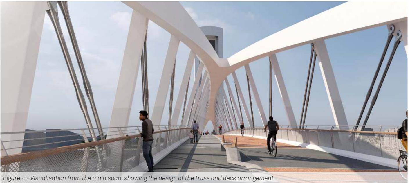
Figure 4 - Visualisation from the main span, showing the design of the truss and deck arrangement
