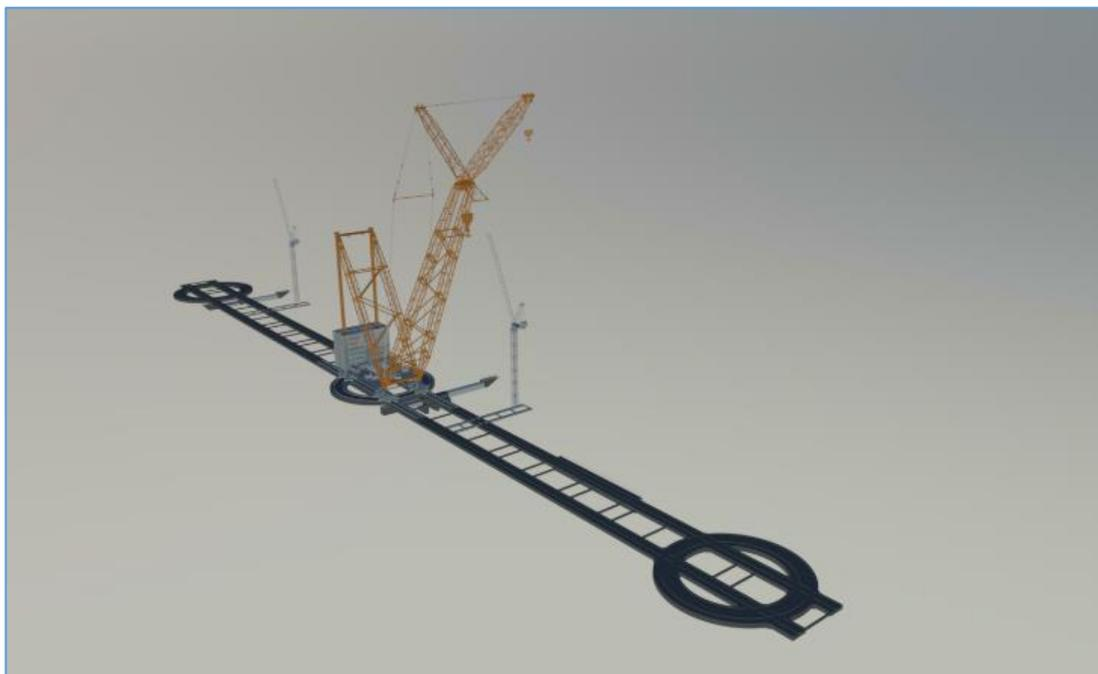
Figure 1 - A model of the crane and the foundation
